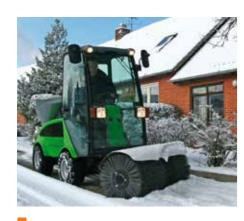
The snow sweeper is perfect for the first snow fall of winter. It will completely remove snow to a depth of 150 mm. The angle, rotation speed and rotation direction can be adjusted from the cabin for the best possible result. The built-in support stand with built-in wheel makes
